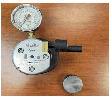
**PULL TEST**Standard: ASTM C1860-21
