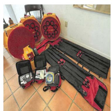
POSI TEST AIR LEAK TESTER Standard: E1186-22
