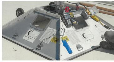
**PULL OFF TEST**Standard: ASTM C1583
